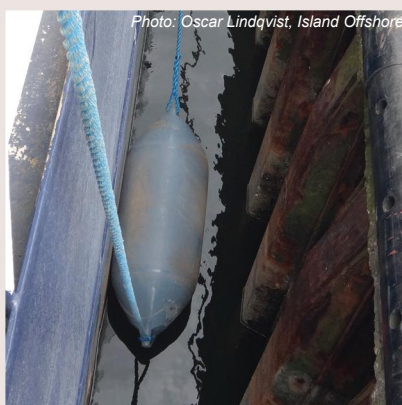
High abrasion resistance and light weight. Resistant to seawater, cleaning agents, common solvents, mineral oil and UV-light. Photos from the vessels Island Patriot and Island Valiant.
